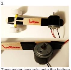
Tape motor securely onto the bottom side of the front of the popsicle stick. This takes a surprisingly long piece of tape.
