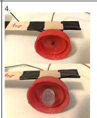
Push a wheel with very small hole drilled into it onto axle of motor. Push glue stick piece on after the wheel to hold it firmly in place.
