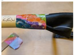
Attach the inner tube to the PVC pipe with duct tape. Wrap tape tightly and make sure no air will leak out.
